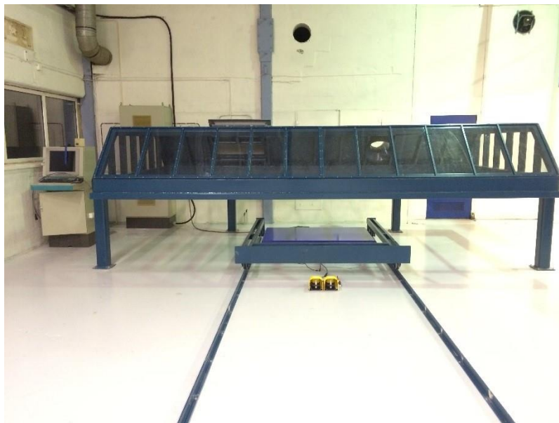
Wind load tester 4,90 m x 2,65 m
